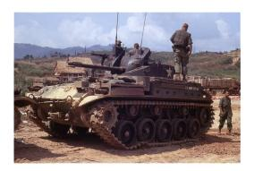
The M42 40 mm self-propelled anti-aircraft gun, or "Duster," is an American armored light air-defense gun built for the United States Army from 1952 until December 1960, in service until 1988. Production of this vehicle was performed by the tank division of the General Motors Corporation. It used components from the M41 light tank and was constructed of all-welded steel.
